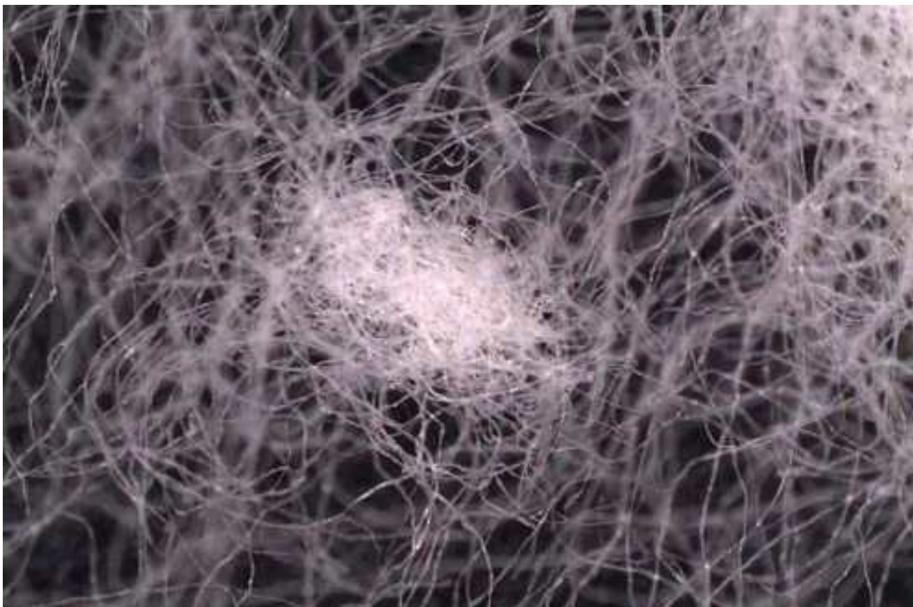
Growers need to consider the impact of management on fibre quality as well as yield. Image of a process nep (an entanglement of fibres which can affect finished fabric). Obtained by means of a Wild Makroskop M420 microscope equipped with a Leica DFC290 digital camera. (Photo: CSIRO)
