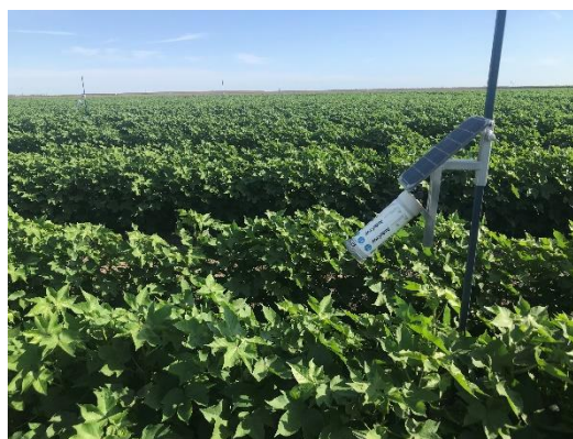
Figure 2: Infrared canopy temperature sensor monitoring crop stress in an irrigated cotton field
